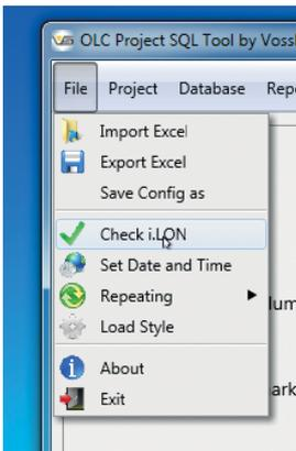
Click on "Check i.LON" in the "File" menu option, after which a window will open with a "Check SmartServer" button and an entry field for the SmartServer's IP address. While it is possible to change this IP address, this usually makes little sense since it would have been automatically taken over from entries made earlier.
