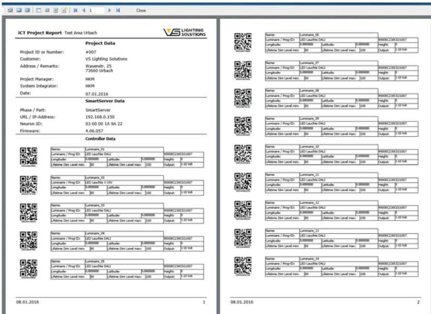
The QR code contains the neuron ID and can be read using commonly available scanners. The last page also contains an overview of all luminaires within the system and/or associated driver data.
