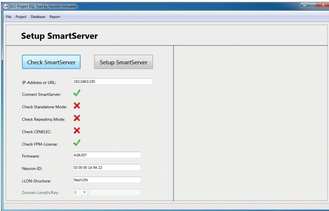
As you can see, the SmartServer is not in the correct mode, which you can now change by clicking on "Setup SmartServer". In addition to changing the modes, you will also have to import various files that are required for further configuration steps. After changing modes and copying the necessary files, a reboot will be needed, which will take several minutes. A progress bar will be displayed throughout:
