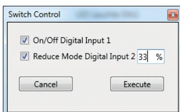
If only the first option is checked, a signal applied to digital input 1 will merely switch light on or off. If the second box is also checked, lighting levels can also be dimmed down to a pre-defined level. Clicking on "Execute" activates the process, which takes no more than a few minutes to complete.
