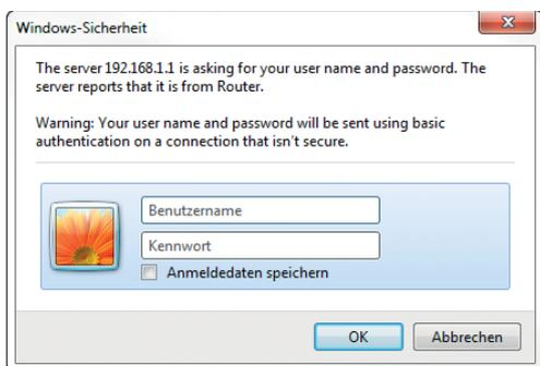
Default settings for user name and password are "root". The router portal then opens with a message that the password needs to be changed:
