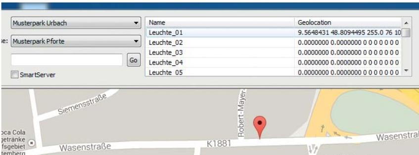
The determined coordinates are then transferred directly to the controllers saved in the databank when "Save" is clicked.
