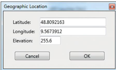
Latitude must be entered in the first row and longitude in the second. The elevation of the device is entered in the third row, but this value has no effect on determining the geographical location. The values are saved by confirming "OK".
