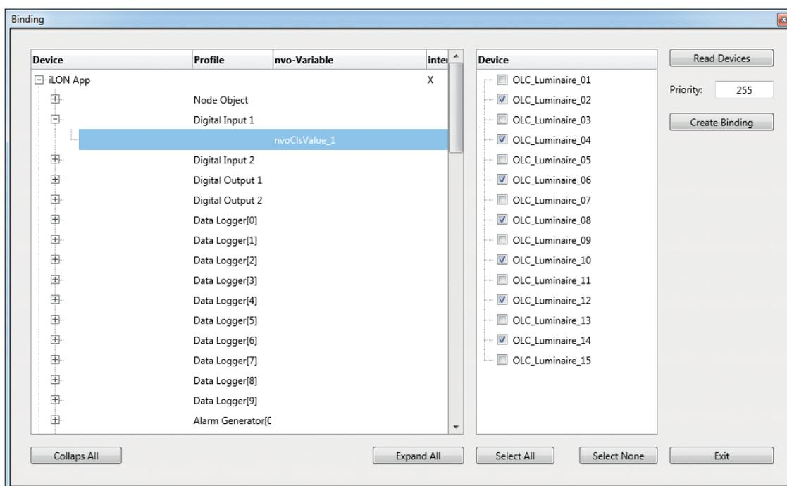
As can be seen, the digital input's output variable (nvo variable) affects the marked controllers. Whether a variable is generated internally by the SmartServer or stems from another external device is shown by an "X" in the "Internal" column.
