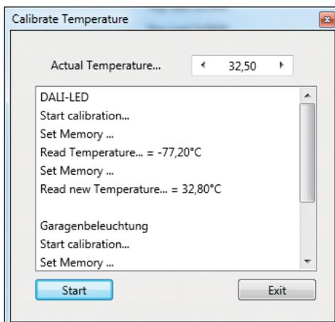
Once the process has been started by clicking on "Start", corresponding information will be displayed. During this process, the internal calibration memory will be set to 0 and the temperature measured (in our example:  $-77.20^\circ\text{C}$ ). Subsequently, a new correction value will be calculated using the target temperature and entered. To finalise, the temperature is measured again. However, this can slightly deviate from the preset value for reasons inherent in the system.
