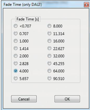
16 different fading times are available for selection. These values cannot be modified and correspond to the DALI standard.
