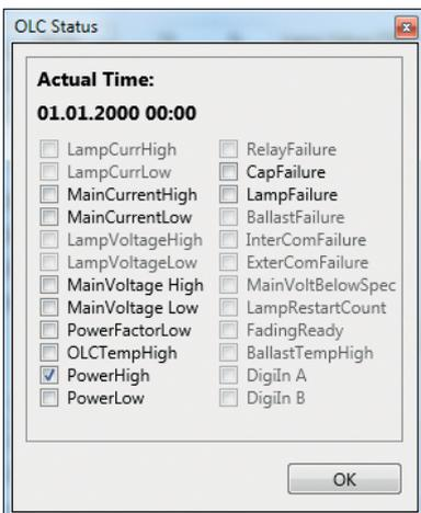
As can be seen in the example, the last transfer took place at 24:00 hours on 01.01.2000 and excessive power consumption was evidently detected. In the following, only those errors displayed in bold type will be explained.
