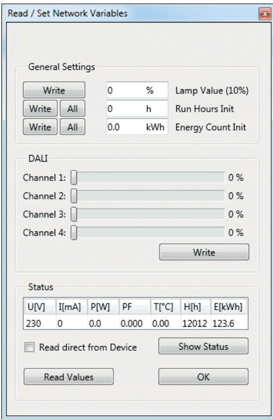
The screen provides an immediate overview of the device status and data can be transferred at the same time, for which the upper three fields are provided. After entering a value, it is then transferred by clicking on "Write". Values entered in the second and third lines can also be transferred simultaneously to all controllers to set initial values.
