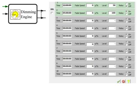
Switching times and dimming levels for normal operation are set in Dimming Engine 1. Times must be entered chronologically. A fade value, a dimming level and a switching state for the two-way relay can be entered for each switching time.
