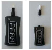
1.2.2. Turn the switch on the top of the iCTI to OFF/USB
