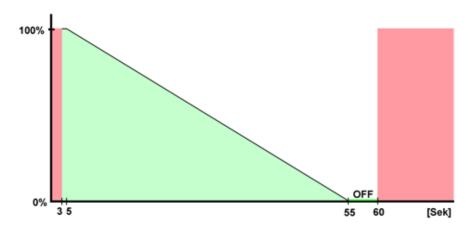
Under 5 seconds: no switching operation Longer than 5 seconds, but under 55 seconds: switches the relay on The dimming values shown below are set in line with the duration of the impulse (between 5 and 55 seconds): 5 seconds: 100% 30 seconds: 50% 55 seconds: 5% or respective linear values in between 55–60 seconds: the relay is switched off 60 seconds or longer: no switching operation
