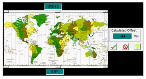
The time zone is set via the upper slider, geographical longitude via the lower slider.
