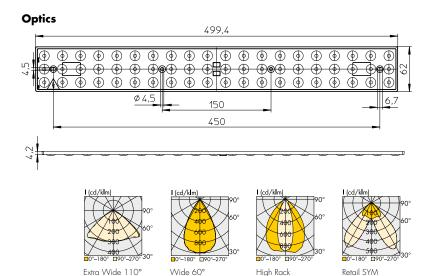
Light distribution curves are preliminary, they are based on simulation. Data are available in .ldt format for download under www.vossloh-schwabe.com.
