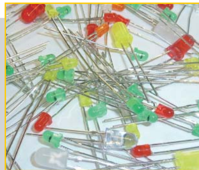
Light emitting diodes in multi-coloured plastic casings
